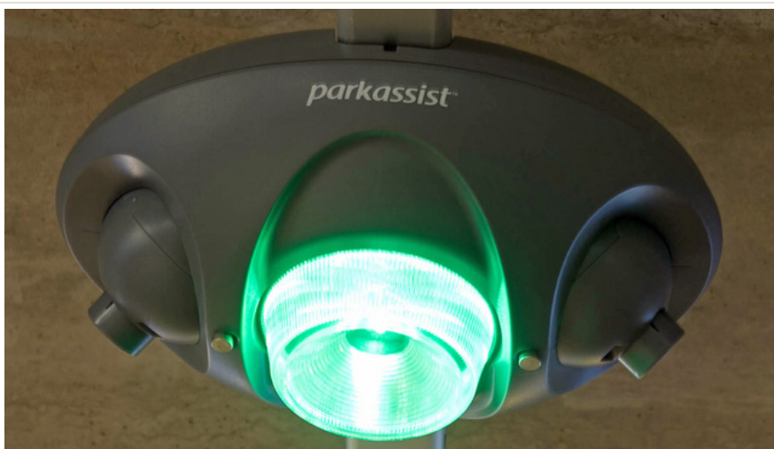
This is one of hundreds of small computer systems that help guide parkers to a free spot. Source: The Australian
